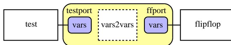
Figure 5: Outline of interfacing two `vars` ports
